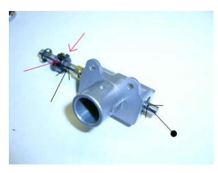
(2) Apply green loctite 290 to the outside wall of a 0425 bearing and insert into the tail box just before putting the tail output shaft assembly into the tail box. Apply a little green loctite to the inside of the 0427 gear before positioning it over the flat spot on the 0541-8 t/r shaft.
