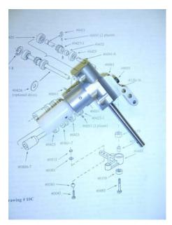
(7) This is the final assembly. I put a little more grease in the tail box just before putting the 120-16 bellcrank support piece on. I used 4707 synthetic hydrocarbon grease, but there are plenty of other kinds that work!
