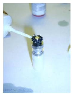
(6) Apply grease to the input 0427-1 gear before final assembly. Smooth it down to a very fine layer with your fingers and then fit the input assembly into the tailbox and do the final fitting.
