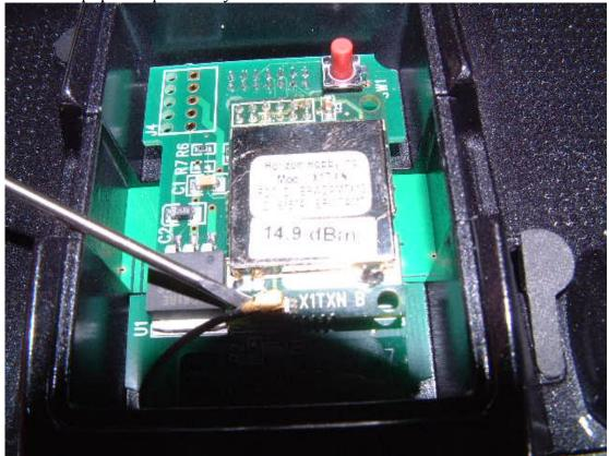
The PCB can now be removed from the case; this comes away with little or no pressure.
