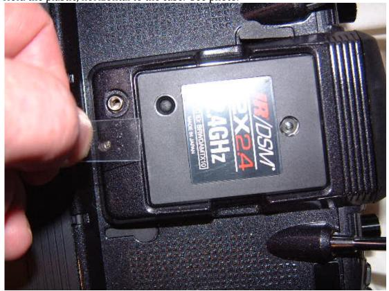
Slide the plastic into the junction of the module cover and the rear cover.
