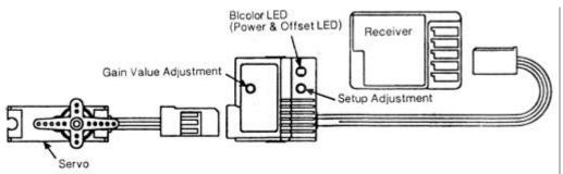
Disconnect the servo to be compensated from the receiver and plug the connector from the gyro there, then insert the servo connector to the gyro port. Be sure to observe the proper polarity on the connector and the gyro port (socket). If the wires on the components are excessively dragged each other, it is not possible to get best vibration absorption with the mounting foam tape, also it may cause possible disconnection during use.
