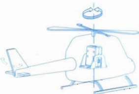
Helicopter (Yaw Stabilization) RX ⇒ PG-02 ⇒ Rudder Servo
