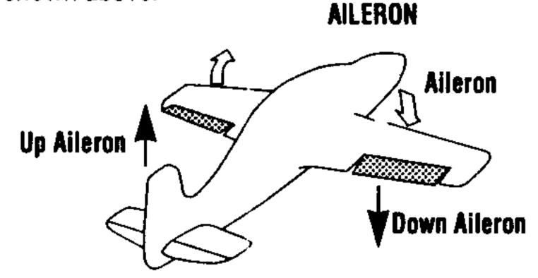
With a quick motion, rotate the fuselage of the model to the right, the ailerons should give a "left control" input as shown above.
