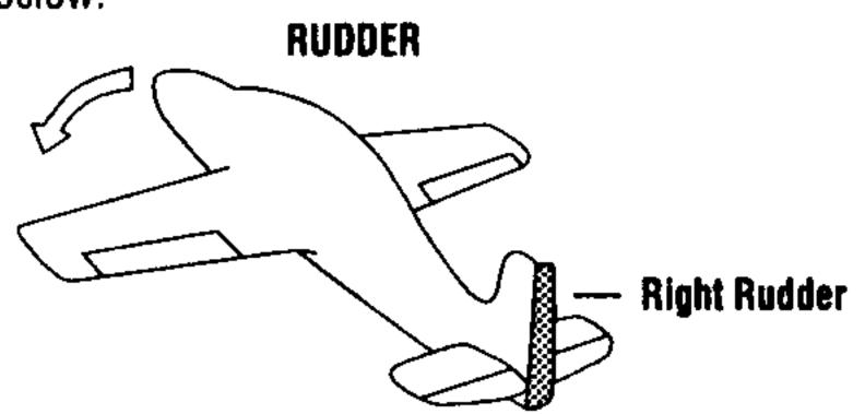
With a quick motion, move the nose of the aircraft to the left, the rudder should deflect to the right as shown above.
