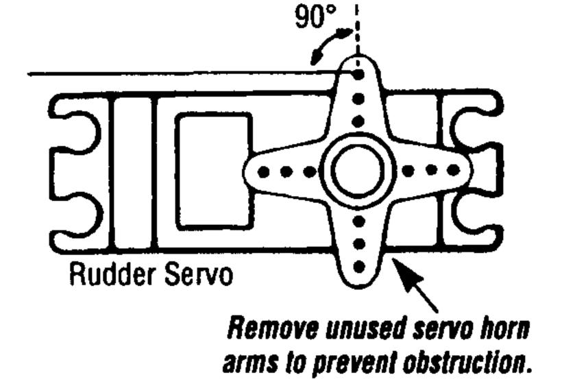
shaft are aligned in such a way that prevents 90 degree positioning of the servo arm. To correct this problem, rotate the servo arm 180 degrees from its original position and reinstall. Once correct alignment has been achieved, secure the servo arm to the servo using the original mounting screw. Next, re-attach the control surface pushrod to the servo arm in its original hole location. Later we will determine the optimum servo arm hole.
