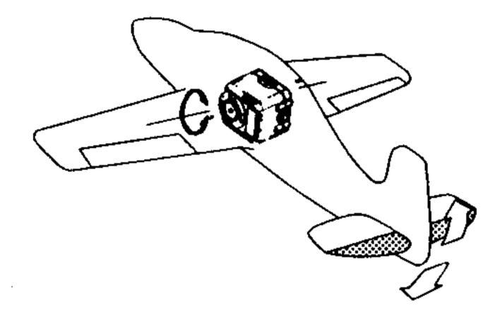
Be sure to thoroughly clean the Sensor/Amplifier mounting area and the aircraft's mounting location with rubbing alcohol prior to attachment. Use one layer of the supplied double-sided tape to secure the unit in place. It is not recommended that "thick" foam tape be used as this could reduce the effectiveness/performance of the NEJ-900 system.
