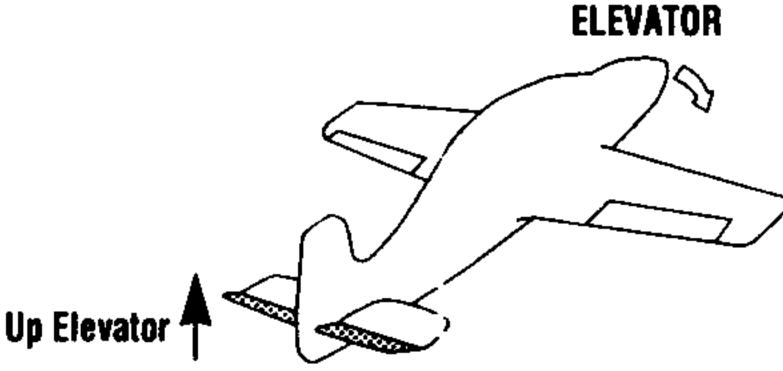
With a quick motion, rotate the nose of the fuselage down as shown above. The elevator should give an "up" control input as shown above.
