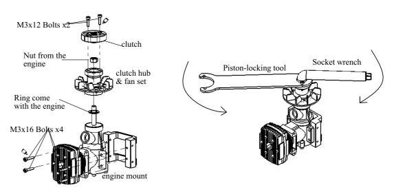
Step 4: Push the whole engine set from bottom of the frames up into the clutch bell. Turn the drive gear when tighting the M3x16 bolts tofix the engine mount on the frames. Adjust the bolts so that the driving gear can turn smoothly.
