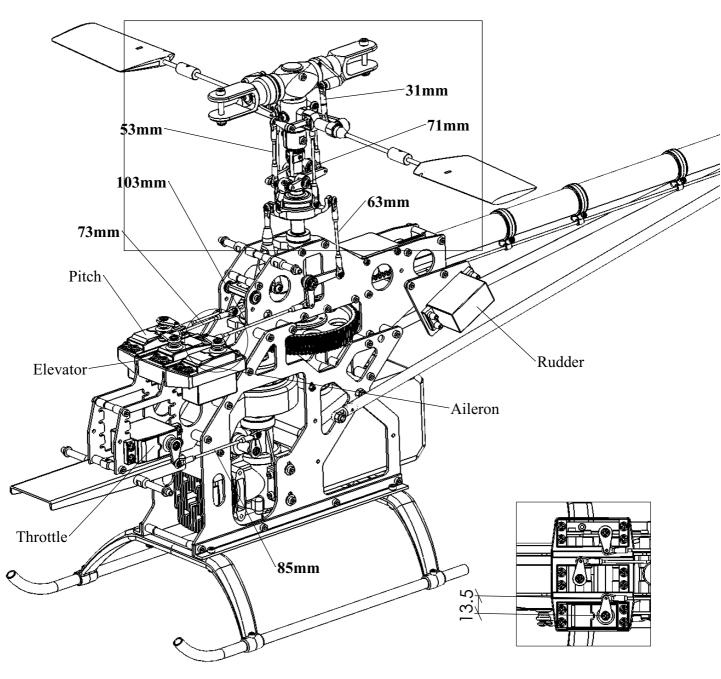
Suggest use the third hole on the horn for Futaba servo. For JR horn, you might need to drill a hole 13.5mm from the center.
