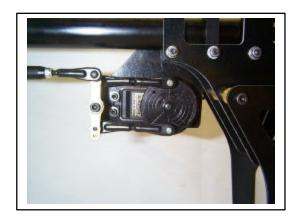
There is a push-pull rudder servo upgrade that completes the push-pull control system offered by Bergen R/C. It includes a dual ball bearing supported arm that transfers the servo loads to the arm. Contact your dealer or Bergen R/C Helicopters for more information.
