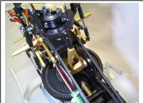
There is an elevator yoke upgrade option available. It consists of a larger elevator yoke and two bearing supported vertical A-type arms to link to the swashplate. The anti-rotation bracket is eliminated and more fluid elevator movement and control is the result. The friction of the anti-rotation bracket and the anti-rotation assembly is eliminated. Contact your dealer or factory about Elevator Yoke Upgrade #280.
